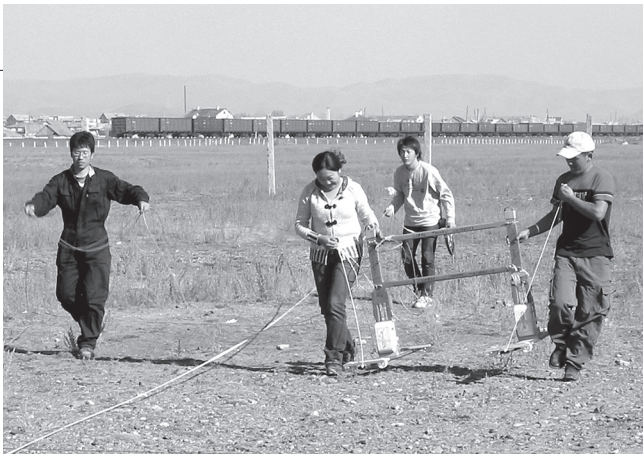
Measuring ground water by GPR (Tuul River, Mongolia).
