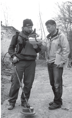
ALIS devices being used to support removal of live landmines in Croatia.
